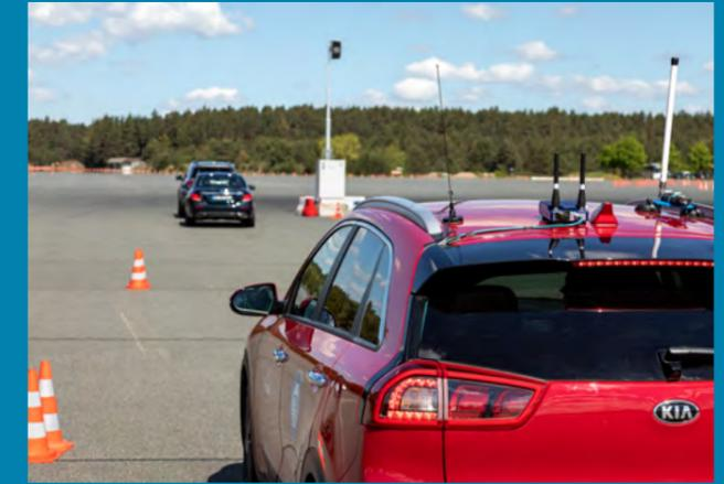
Special robotic cars driving on pre-programmed routes simulate the surrounding traffic
