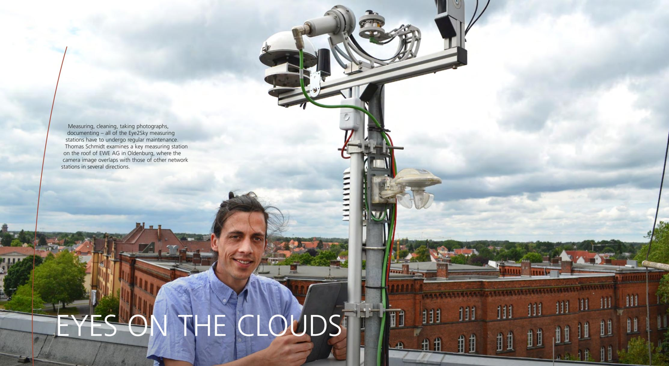
Measuring, cleaning, taking photographs, documenting – all of the Eye2Sky measuring stations have to undergo regular maintenance. Thomas Schmidt examines a key measuring station on the roof of EWE AG in Oldenburg, where the camera image overlaps with those of other network stations in several directions.
