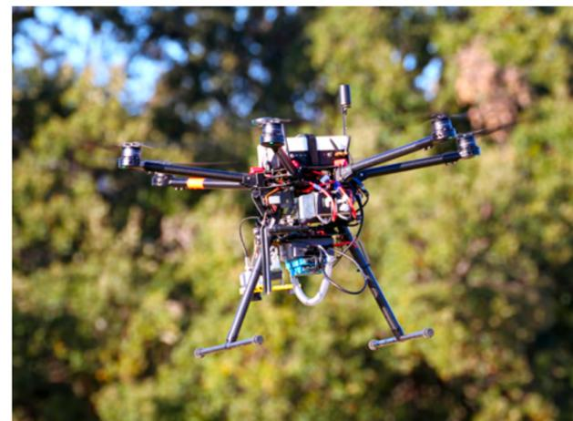
One of the three unmanned aerial systems from the HEIMDALL project, equipped with cameras and thermal imaging sensors.
