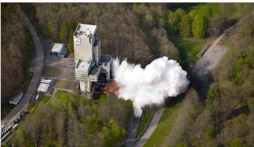
Every test on a main-stage engine is an impressive event. A Vulcain 2.1 consumes 600,000 litres of liquid hydrogen and 200,000 litres of liquid oxygen – forming pure water – during a firing duration of approximately 12 minutes. Together with the water used for cooling, this forms the characteristic steam cloud above the test site. Later, this falls back to Earth as rain.
