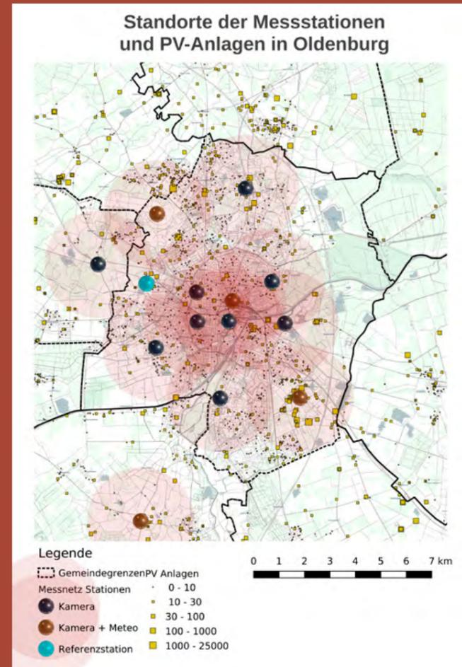
The Eye2Sky network is to be expanded in the Oldenburg urban area in a particularly close-knit way. The need for accurate forecasting is especially pressing here due to the numerous solar units installed on the roofs of private homes.
