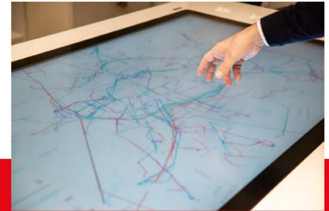
A large touchtable enables users to visualise the data collected by MovingLab. Different colours denote the various means of transport. Filter functions allow specific queries by categories such as age group or the purpose of the journey.
