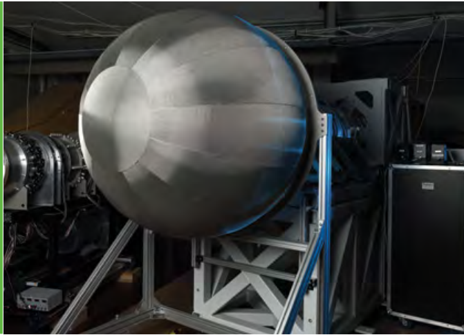
New propulsion concepts can be tested as early as the prototype stage on the CRAFT test stand at the DLR Institute of Propulsion Technology in Berlin.
