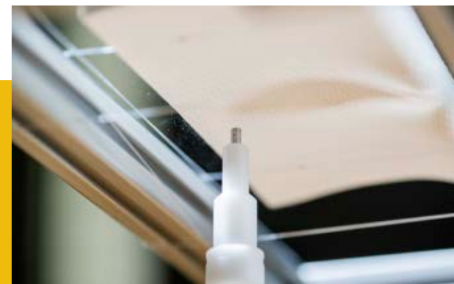
A projectile taps the component and causes it to vibrate
