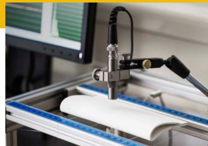
A microphone records the sound of the vibrating blade model
