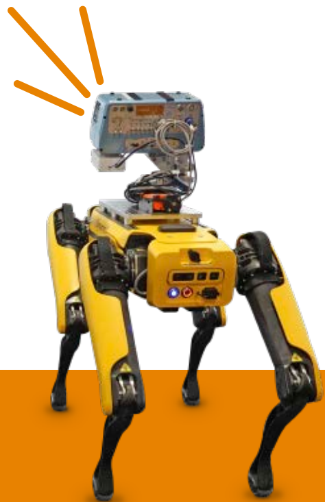
DLR's Integrated Positioning System (IPS DLR OS), here carried by Boston Dynamics robotic dog SPOT, measures the interior building and room geometry.
