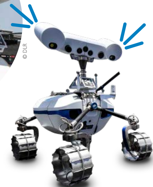
The final preparations at Base Camp on Mount Etna before robot LRU1 starts its mission. Several camera systems are mounted on its head. With the exterior filter wheels it recognises different frequency ranges.
