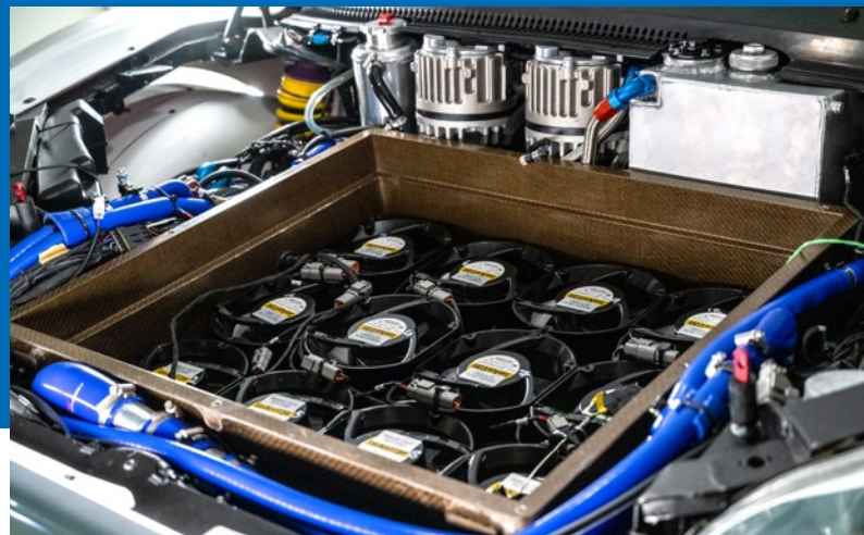
A look under the bonnet reveals the supporting fans of the tyre particle extraction system
