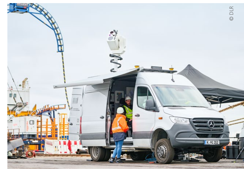
Observational instruments are installed on a van so that they can be deployed quickly and flexibly at the site of operation
