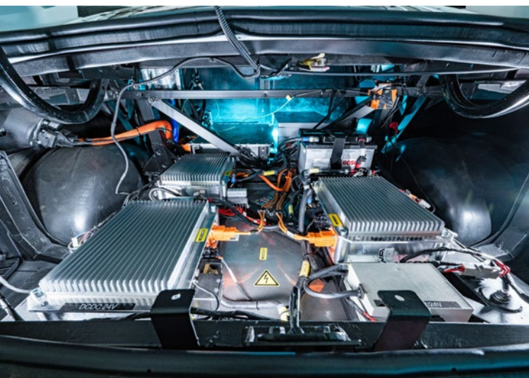
The battery, the power electronics and the DC converter for the power supply are installed in the rear of the vehicle.
