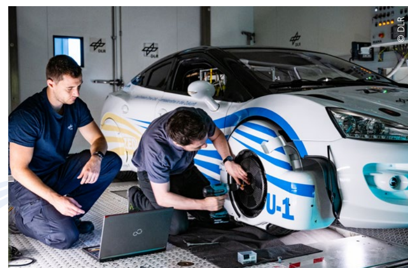
Fabius Epple and Sven Reiland from the DLR Institute of Vehicle Concepts, both members of the ZEDU team, mount the fairing on the measuring wheel
