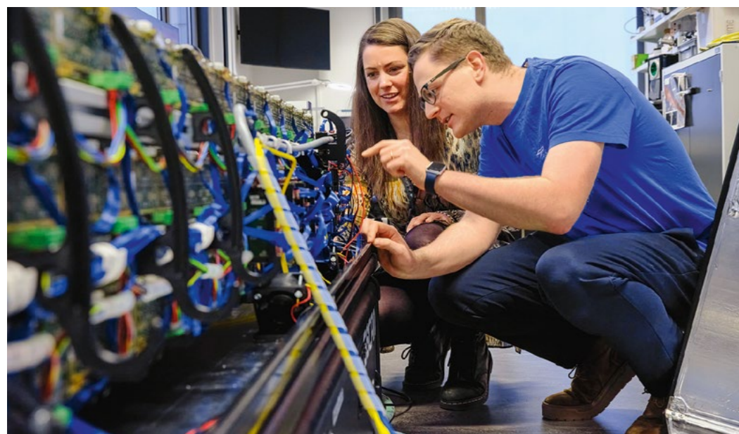
Sarah Barnes and her colleague Maximilian Pérez Prada investigate the readout electronics of the muon detector.
