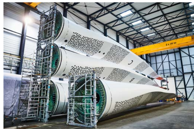
The rotor blades are each 57 metres long and weigh approximately 20 tonnes
