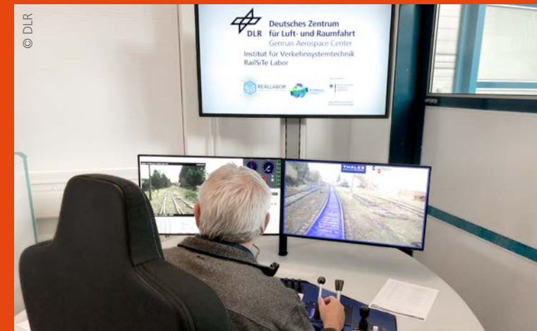
The train driver in Braunschweig controlled the train in the Ore Mountains via 5G
