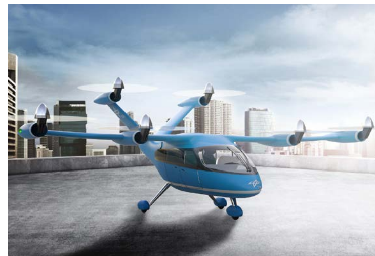
Design of a tiltrotor air taxi with six swivelling rotors
