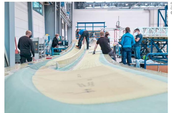
The team tests the installation of the sensors on the rotor blades at the DLR Center for Lightweight-Production-Technology in Stade
