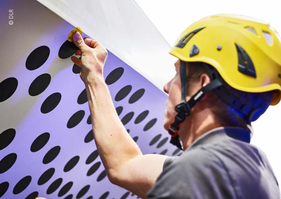
Yves Govers from the DLR Institute of Aeroelasticity checks the measurement markings on one of the rotor blades
