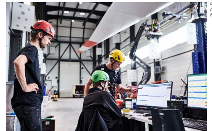
Before assembly, all six rotor blades were dynamically measured by the experts at the DLR Institute of Aeroelasticity. In addition, one blade was statically tested in collaboration with Fraunhofer IWES.
