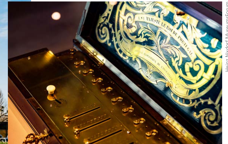
The Thomas Arithmometer. This sophisticated version of the calculator was a gift to the King of Portugal.
