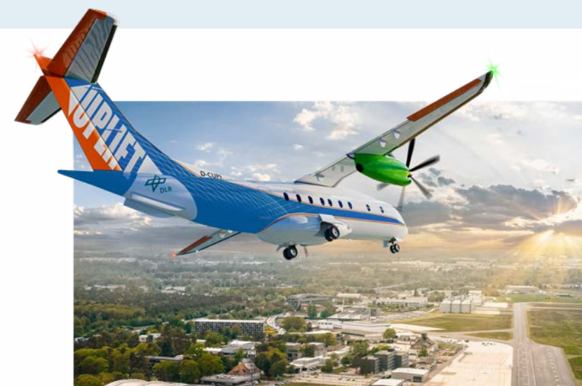
Following conversion into a flying laboratory, the newly acquired aircraft Dornier 328-100 Model 20 will be used for research into hydrogen technologies for aircraft, among other things.
