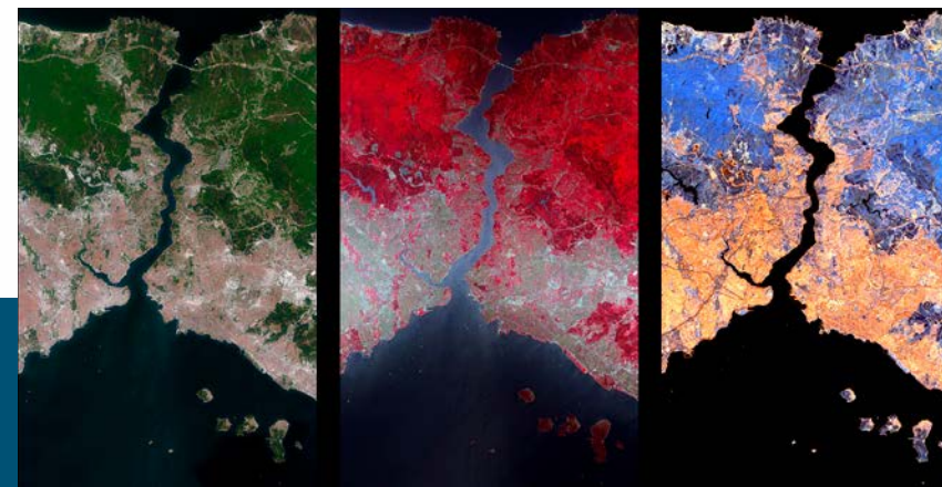
The Environmental Mapping and Analysis Program (EnMAP) is the first German hyperspectral satellite mission. Using its two spectrometers, it analyses the radiation reflected from Earth, ranging from visible light to short-wave infrared, at a hitherto unparalleled spectral resolution. These images show the Bosphorus in Turkey. On the left is a true-colour representation; in the centre, differences in vegetation become clear in the near-infrared range; on the right, soil and rock features can be distinguished.
