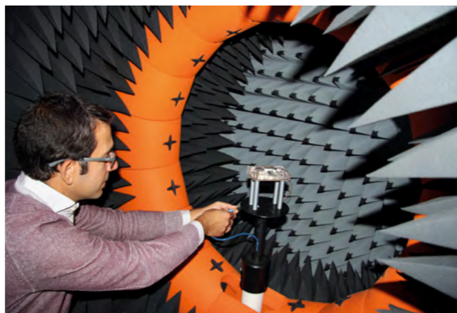
Stefano Caizzone from the DLR Institute of Communications and Navigation in Oberpfaffenhofen tests a '3+1 antenna'. This antenna is specially designed for receiving satellite navigation signals on board civil aircraft and is robust against both jamming and spoofing.
