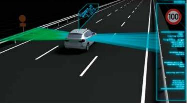
Positioning of an autonomous vehicle within the lane of traffic. The 'DriveLines' (crash barriers as well as the lines with the lane markings) are incorporated in the map with their exact coordinates. The traffic sign serves as a 'landmark' in order to safeguard the vehicle's position once again.
