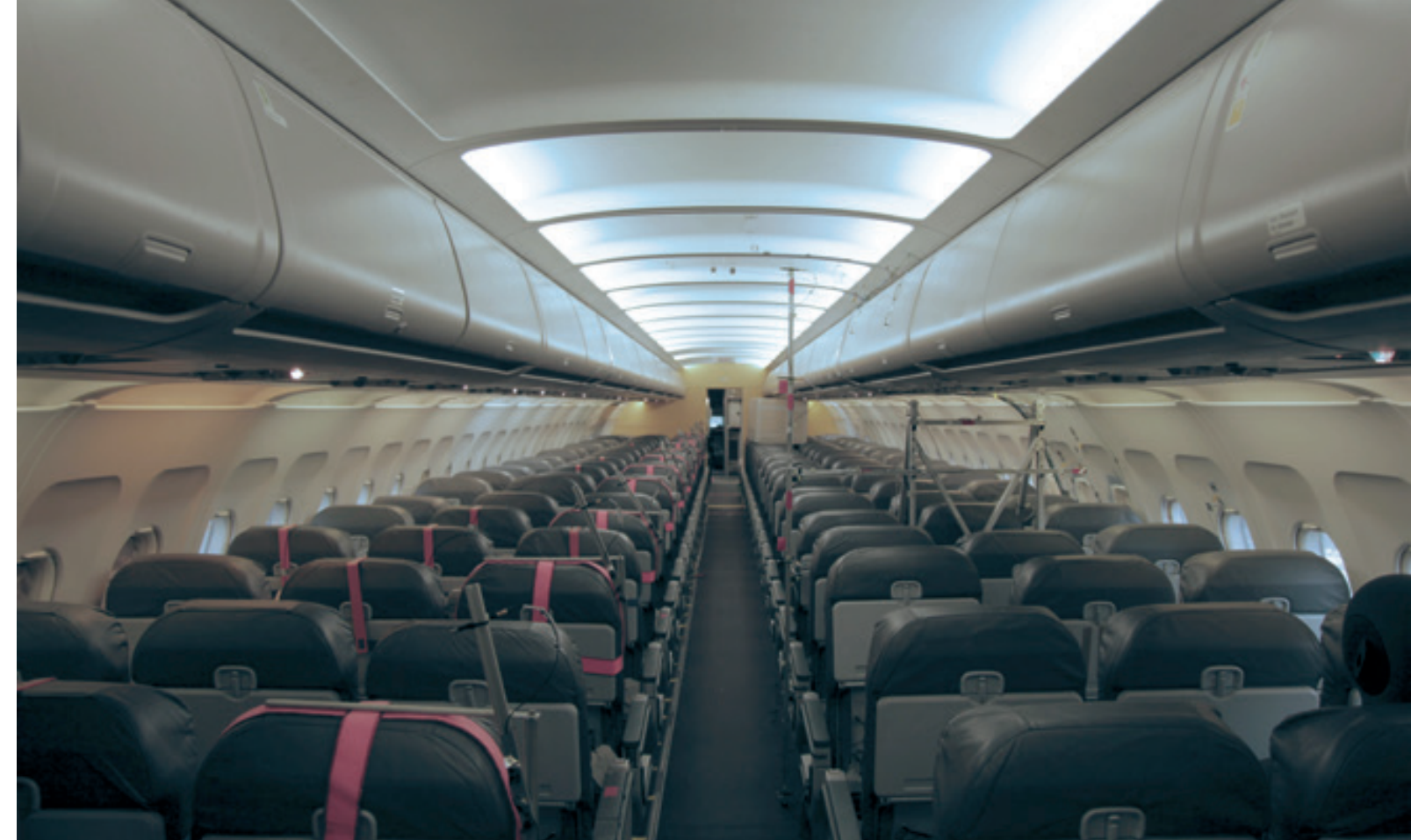
Measurement section of the cabin equipped with static microphones. Acoustic separation from the remaining section of the cabin using a foam partition.
