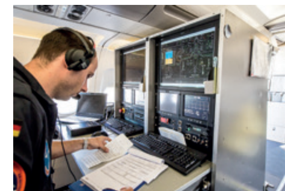
The basic measurement system in the ATRA cabin. The flight experiment data are pooled here
