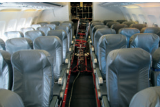
Microphone array that can be moved longitudinally during flight to measure noise pressure and frequency at various cabin positions
