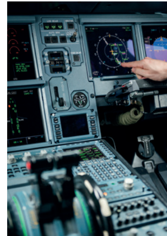
Using satellite navigation and the latest aircraft systems, curves with fixed radii between two waypoints can be accurately planned and curved approaches flown with high precision.
