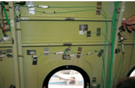
Installation of acceleration recorders on the exposed outer skin of the ATRA aircraft structure
