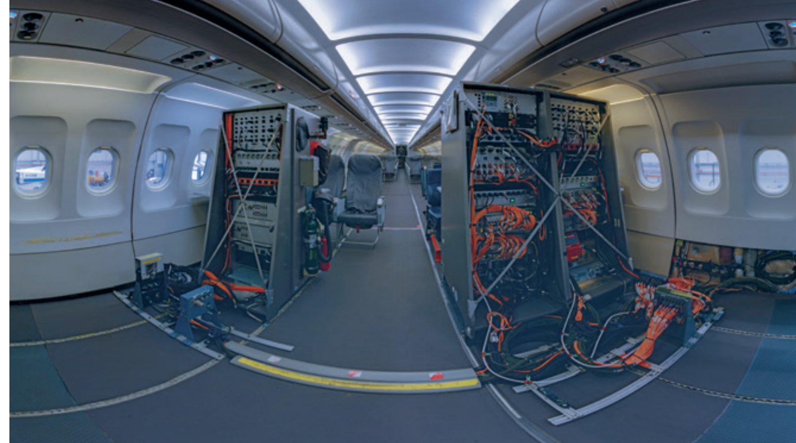
Panoramic view of the aircraft cabin. The front rows of seats in ATRA have been replaced with the basic measurement system, which enables a vast range of research and mission types
