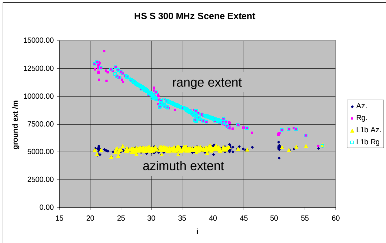
Fig. 2-6: Measured scene extent of High-Resolution Spotlight products in single pol 300 MHz mode for different scene center incidence angles ( i ) taken from the commissioning phase product characterization report.
