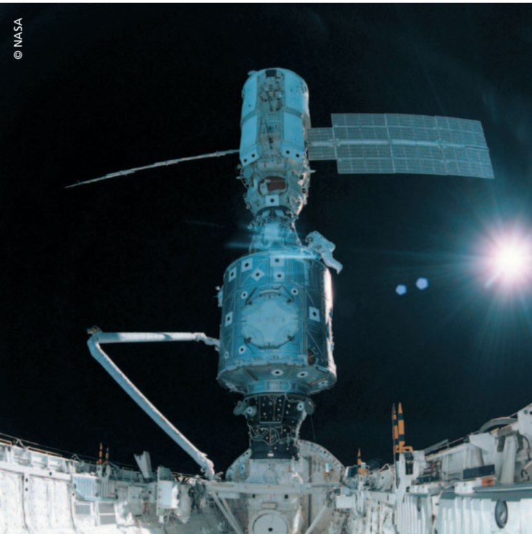
In December 1998, the crew of STS-88 began active construction of the ISS. This image shows the docking of the US-built Unity module with the Russian module Zarya. Sergei Krikalev was on board.
