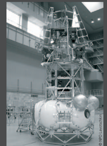
The Phobos-Grunt spacecraft, built by NPO Lavochkin in Moscow. A return capsule will bring samples from Phobos to Earth in 2014.
