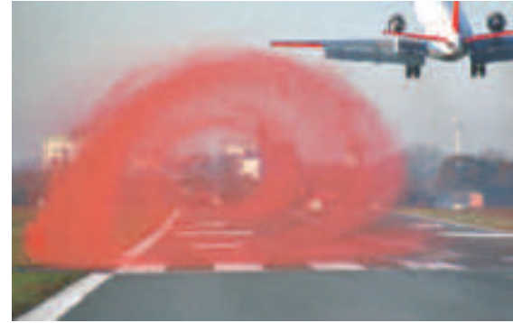
The vortex of the ATTAS, shown here during take-off of the VFW 614, was measured for the first time using a LIDAR from another aircraft (Falcon)
