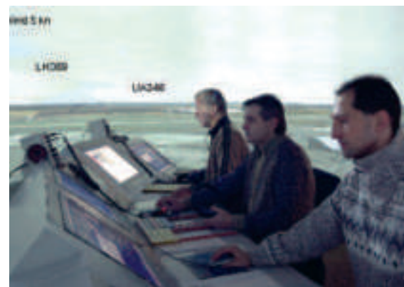
Top: Augmented vision experiment at the Dresden tower with transparent holographic projection to overlay the weather data on the outside view; bottom: Control center with reconstructed outside view (right) using the example of the 300° tower simulator visual system as an augmented tower vision experimental environment (with integrated flight numbers)
