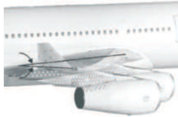
Curvature and torsion on the aeroelastically deformed wing
