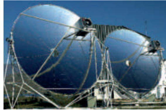
Dish/Stirling prototypes during testing at the Plataforma Solar de Almeria
