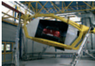
The dynamic driving simulator makes near realistic testing of assistance systems possible
