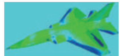
Pressure distribution over the entire model surface is detected using pressure sensitive paint on an EADS-MAKO model in the DNW high-speed tunnel
