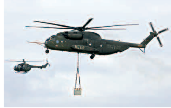
CH-53 G transport helicopter being tested with 4 tons of underslung load; Bo 105 light helicopter of the Federal Army
