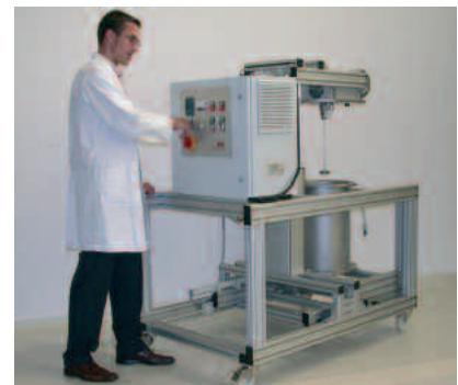
Microwave resin heater for process acceleration
