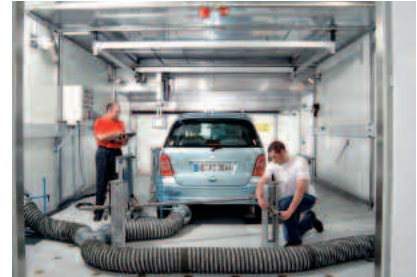
A fuel-cell concept vehicle being tested at the all-wheel rolling test bench with exhaust gas analysis and climate control at the Institute of Vehicle Concepts, DLR Stuttgart
