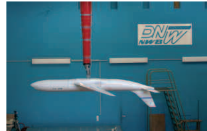
The system is capable of simulating with a high degree of precision not only all rotation movements of the model around its axes but also lifting and flapping motions
