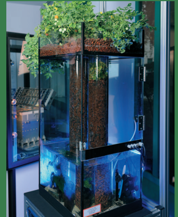
The core of the C.R.O.P. life support system are the tubes, each filled with lava rocks. Bacteria consume waste in the tubes. The metabolic products are a valuable source of nutrients for the plants.
