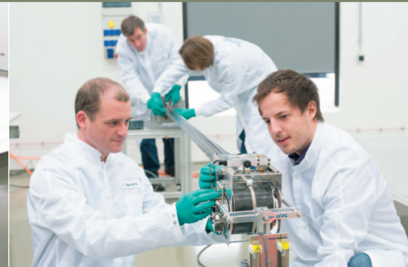
A sophisticated mechanism to unroll the mast in microgravity. In the integration hall in Bremen, the researchers test the smooth operation of this technique.
