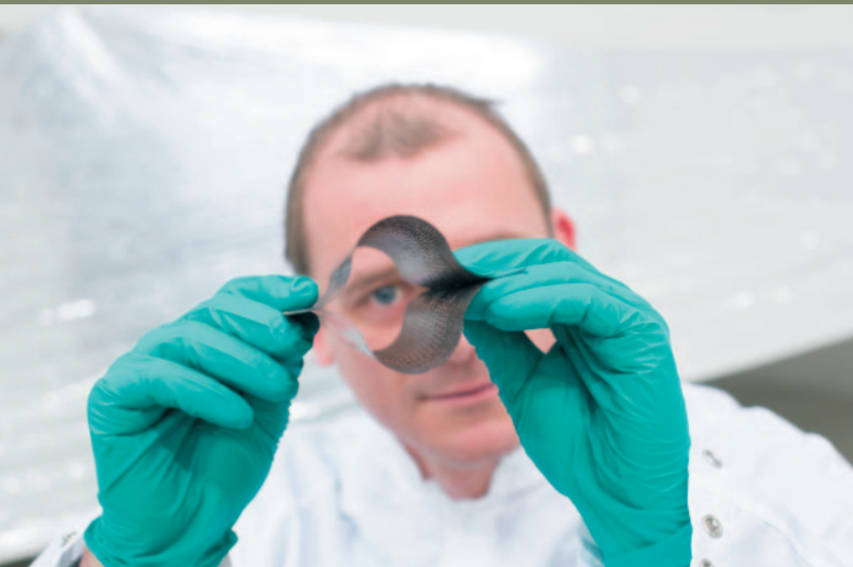
The masts that support the sails during flight must be both strong and flexible. Tom Spröwitz, Head of the System Conditioning Department at the DLR Institute of Space Systems knows that carbon fibres impregnated with liquid resin are suitable.
