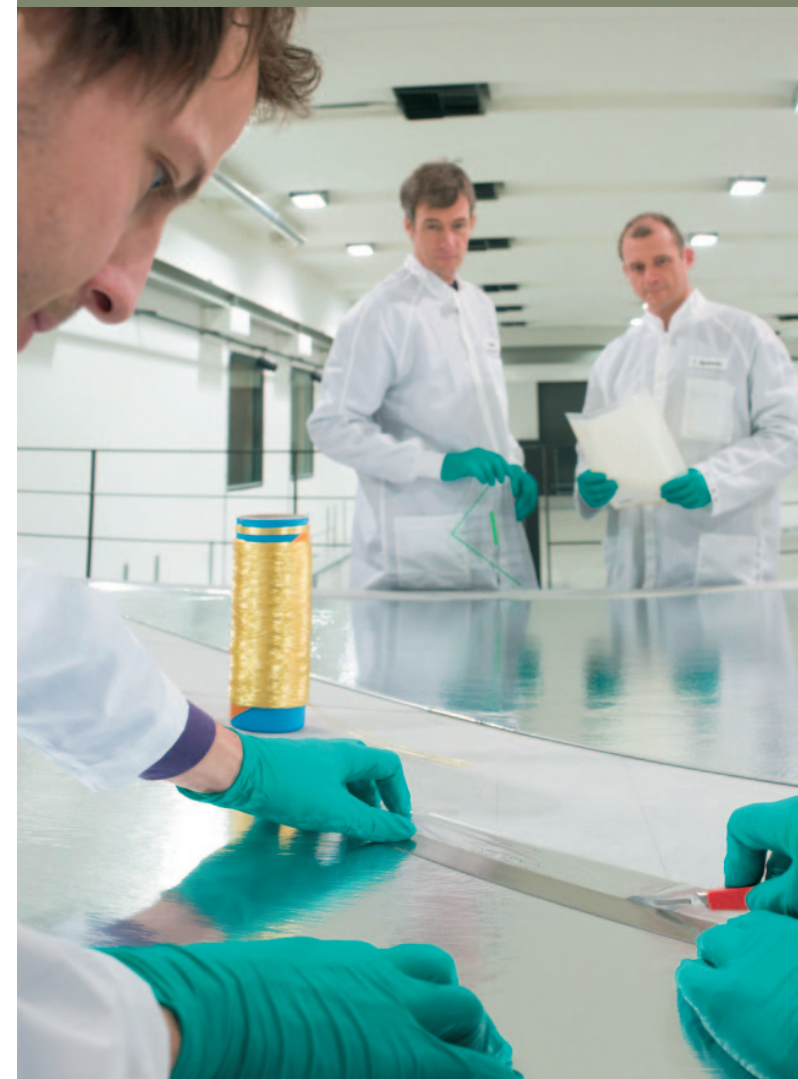
On the suction table, the team cut and glue the delicate film to create the sails. A thread in the outer edge then ensures that the deployed sail will have the correct tension.
