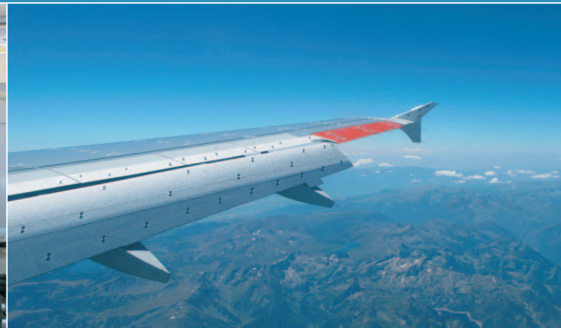
Starboard wing with deformation markers and specially patterned foil during a test flight over the Pyrenees
