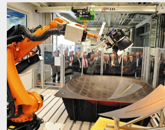
The robot with the laying head has an especially large range for picking up and depositing the thermoplastic sections
