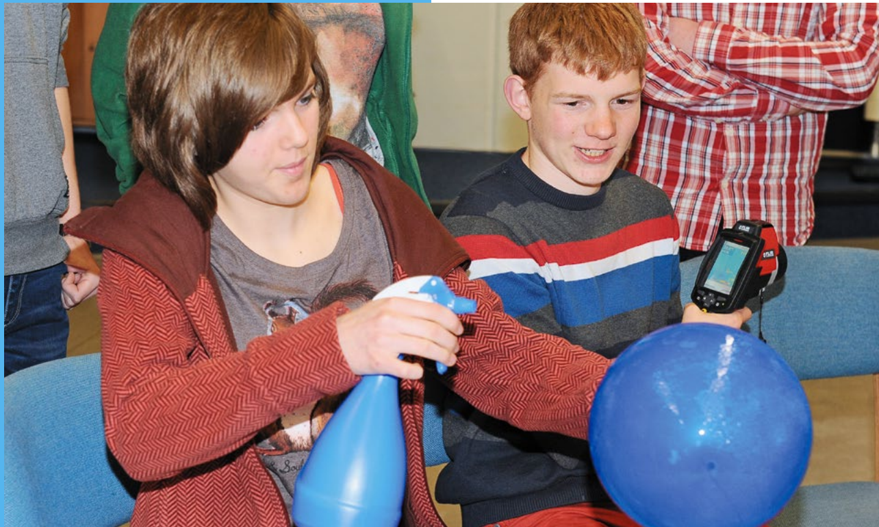
The balloon is sprayed with cold water. Using the thermal imaging camera, Jan-Niklas can then reveal how the energy is distributed over the surface.
