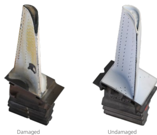
After many long-distance flights, sections of the white ceramic thermal barrier coating on the left blade have spalled.
