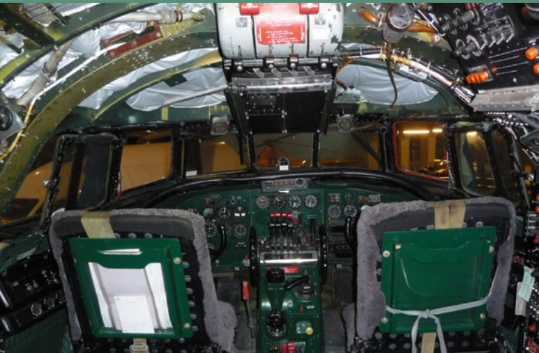
Cockpit of the four-engined Lockheed L 749 'Constellation' long-range airliner, a precursor of the later and very popular 'Super Connie'. Numerous circular analogue gauges dominate the image. Just visible on the right is the flight engineer's console.
