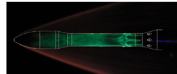
To record the variations in the air flow, engineers placed a film of oil on the model of the Vega rocket. The images show how the oil particles are distributed when subjected to various experimental conditions.
