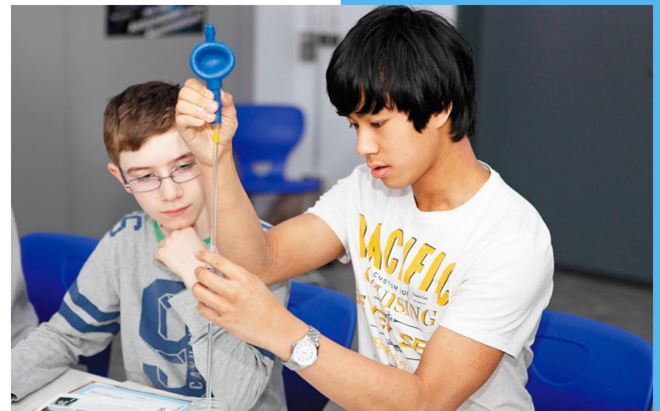
Revealing the secret of the Grätzel cell – Nguyen takes a few drops of titanium dioxide solution and applies them to small thin glass slides. A flow of current is established between the joined glass slides.
