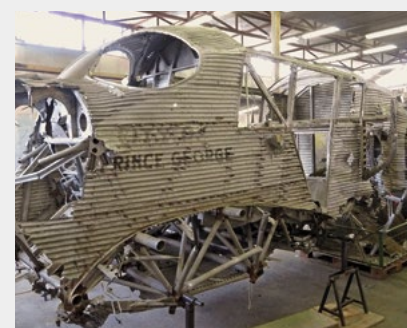
The Canadian Junkers F 13 'City of Prince George' is the template for reconstructing a working model of this type.
