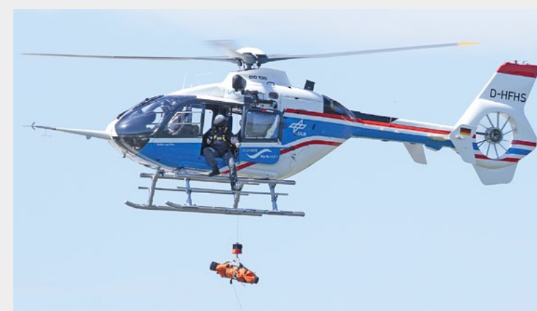
The DLR EC-135 ACT/FHS (Active Control Technology/Flying Helicopter Simulator) research helicopter carrying out a flight test with an external load on the rescue winch
