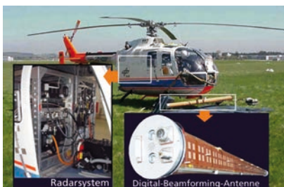
Digital beamforming demonstrator on a DLR helicopter
