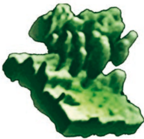
Demonstration of tomographic imaging of a group of trees in L-band. In this example, the radar data were recorded using DLR's airborne SAR system by making several passes at intervals of a few minutes.
