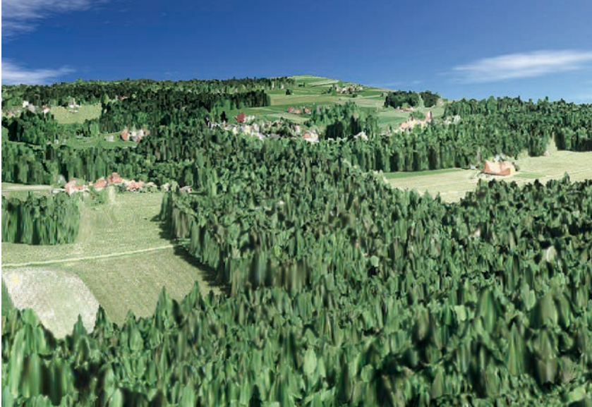
3D representation of the Stadtwald forest in Traunstein, Germany. The forest height was derived from radar data using polarimetric SAR interferometry.
