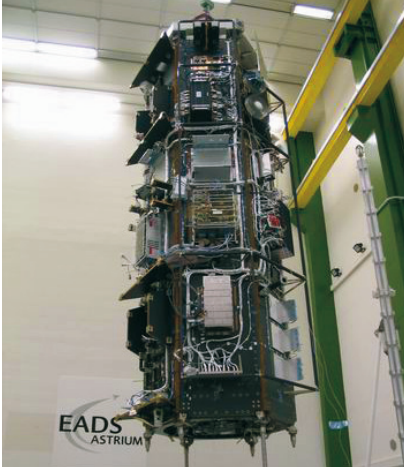
Integration of TerraSAR-X at Airbus Defence and Space (previously EADS Astrium GmbH) in Friedrichshafen, Germany
