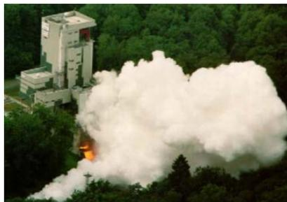
Test facility P5 running the Vulcain 2 engine @ 46 kg H<sub>2</sub>/sec
