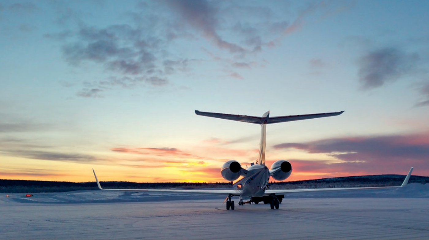
HALO shortly before take-off. The atmospheric research aircraft is based on a Gulfstream G550 long-range business jet. The combination of long range performance, the ability to operate at high altitudes, an extensive payload capacity and comprehensive instrumentation makes it a globally unique research platform.
