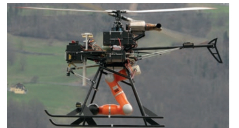
Autonomous Flettner helicopter with integrated robotic arm
