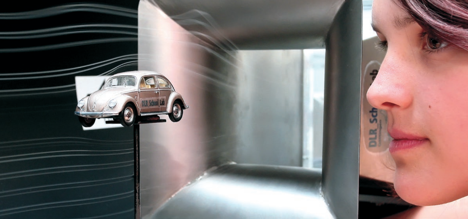
The invisible made visible – wind tunnels reveal the flow around objects placed in them. An image from the DLR_School_Lab in Göttingen illustrates this.
