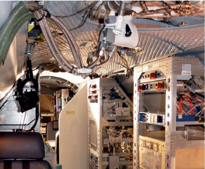
The interior of HALO. There are up to 15 racks for scientific instruments in the cabin. At the front right of the image are two instruments; one for measuring humidity (hygrometer) and ozone. In the background is the airborne mass spectrometer AIMS. It measures halogen and nitrogen oxide compounds that promote polar ozone depletion.
