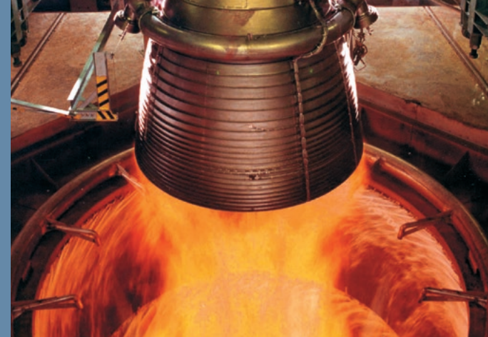
Vulcain 2 engine during a test at the DLR P5 test bench
