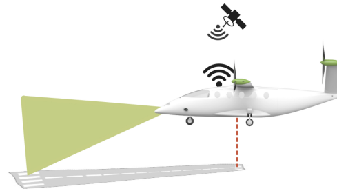
Figure 3.9.: Autonomous systems for landing and height detection: LIDAR (red), radar (green), GPS (black)
