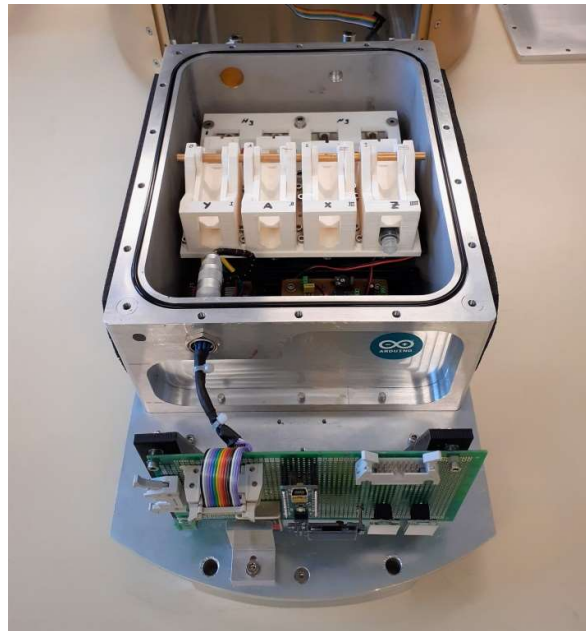
Figure 1: Graviplax experiment insert: four samples with Trichoplax adherens are chemically fixed at defined times during the rocket flight
