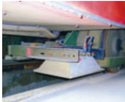
Rail switch recognition for localization using an eddy current sensor under a train
