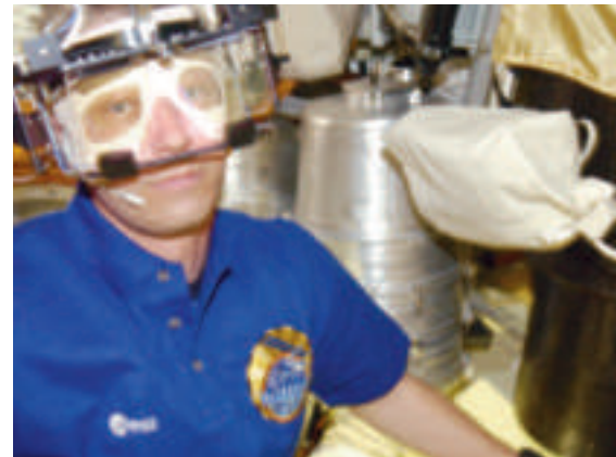
ESA Astronaut Thomas Reiter during the Astrolab mission with a 3D Eye Tracking Device for research of the balance system
