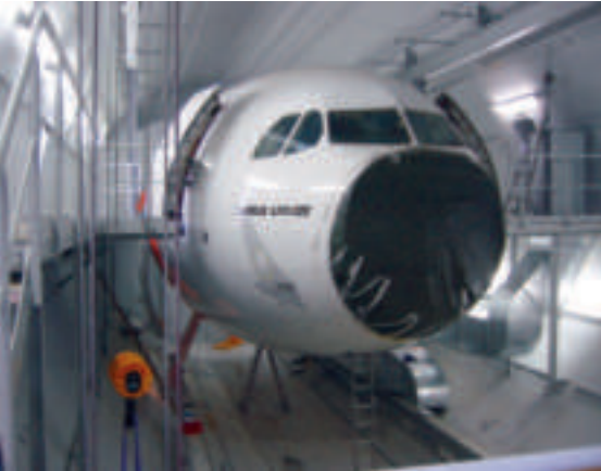
Aircraft torso in the low-pressure chamber
