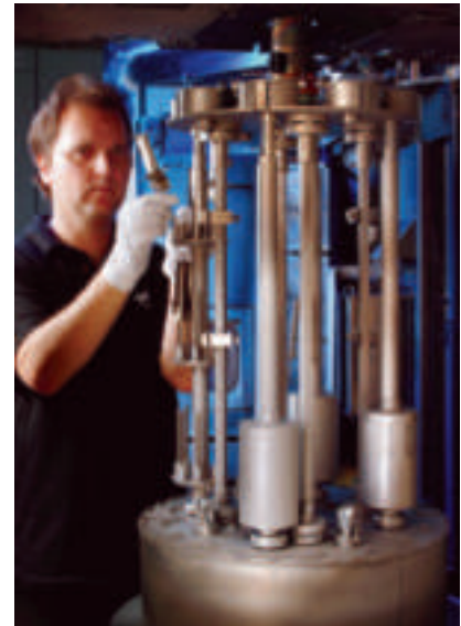
Installation of a turbine blade for coating in the new multi-source magnetron sputtering system (MEGA)
