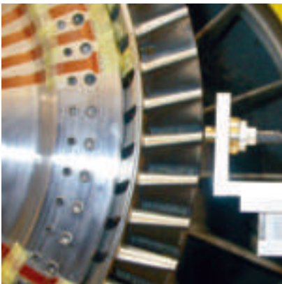
Assembly of the test section: hub contour in the back cascade (top) and control of the blade tip radius after the rotor has been mounted (bottom)
