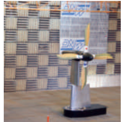
The TILTAERO half-hull model in the wind tunnel
