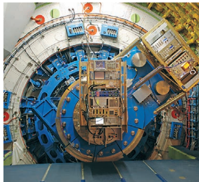
On the reverse side, the remote infrared spectrometer GREAT is mounted on the telescope flange in the pressure chamber. During flight, GREAT moves within a range of plus/minus 20 degrees from the vertical position.
