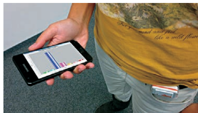
Inertial sensor module (hip) and display of activity on a smartphone
