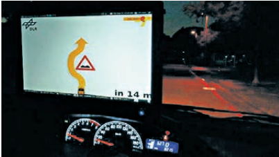
Pothole position and evasion recommendation are transmitted to other vehicles in the area
