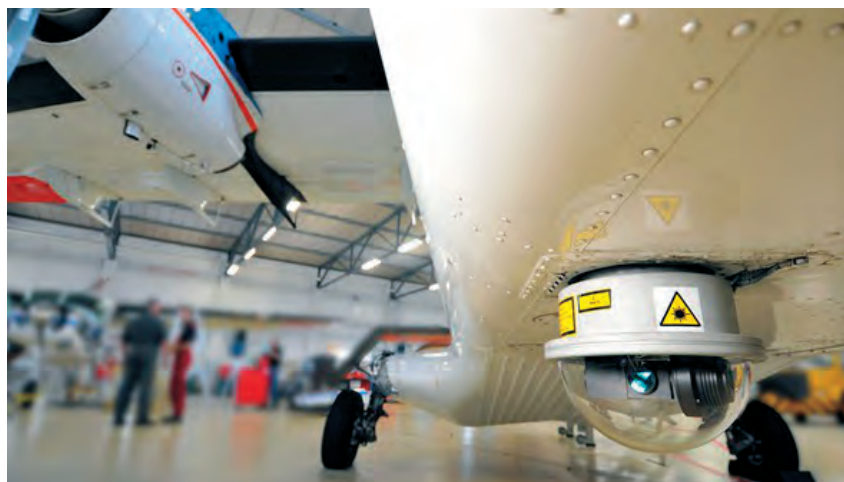
The external attachment of the laser terminal is affixed to the fuselage of the DLR research aircraft DO 228-212
