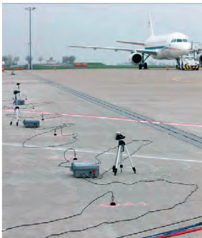
Microphone array and individual microphones for measuring engine flow
