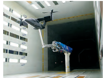
NICETRIP wind tunnel model in the 9.5 metre x 9.5 metre measuring section of DNW LLF
