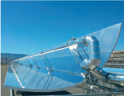
Direct steam generation in parabolic troughs at Plataforma Solar in Spain
