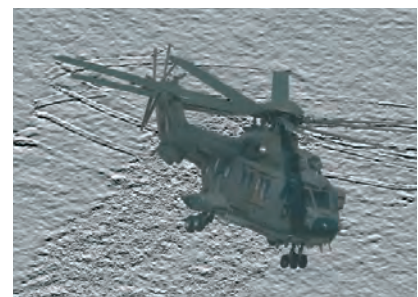
Main rotor vortices on a Eurocopter Cougar helicopter in low-velocity forward flight
