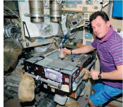
E-Nose electronic gas sensor for detecting microbial contamination on the International Space Station ISS
