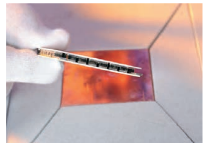
Thermoelectric generator module: transforms excess heat into electric power
