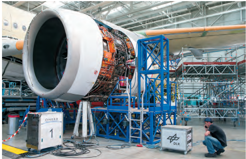
Ground vibration test with Airbus A350 XWB
