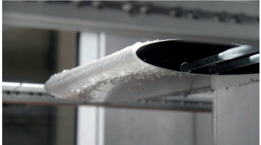
Icing test rig with wing test sample
