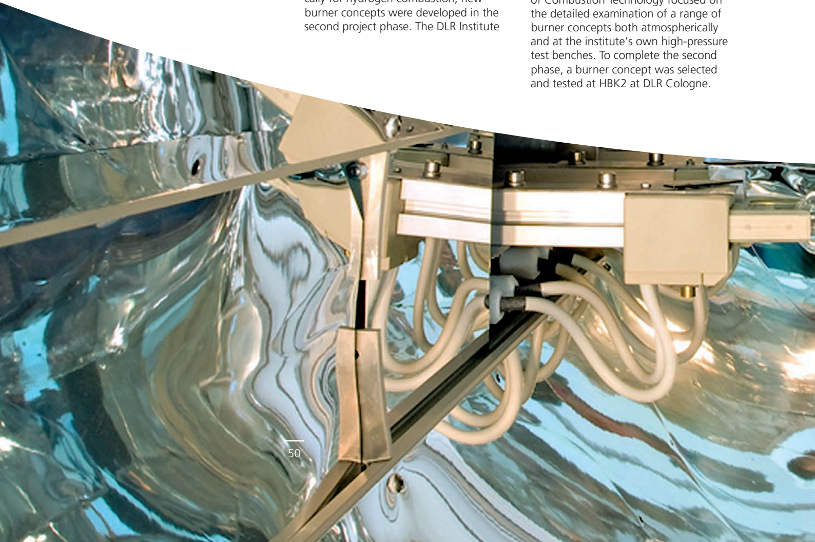
Measuring the flow field of a burner concept optimised for hydrogen using Particle Image Velocimetry (PIV) at the HIPOT (High Pressure Optical Test rig)
