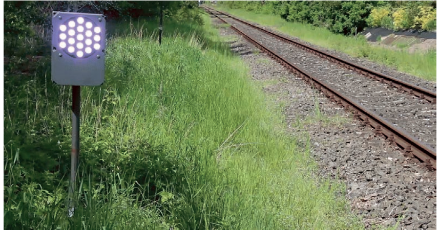
Flashing light at level crossing to guide drivers' gaze
