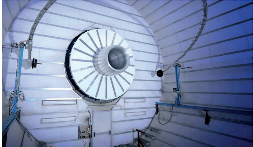
Compressed air reduces engine noise in the absorption chamber
