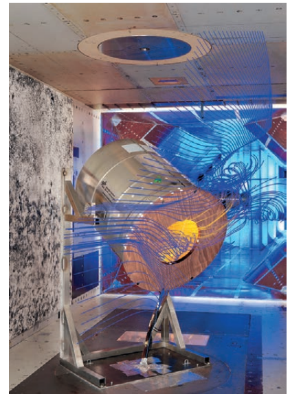
Model of a cavity receiver at the cryogenic wind tunnel in Cologne. The lines identify the wind flow calculated with the help of a computer.
