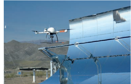
A quadcopter flies past a parabolic trough collector during a test flight at the Plataforma Solar de Almería
