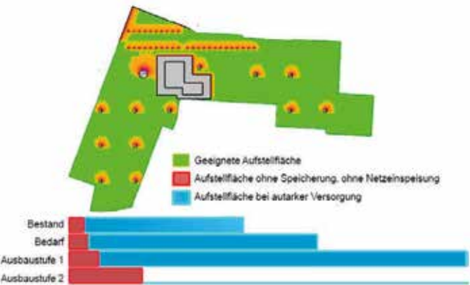
Areas of the Weilheim site with sufficient light exposure to enable the installation of a ground-based PV system
