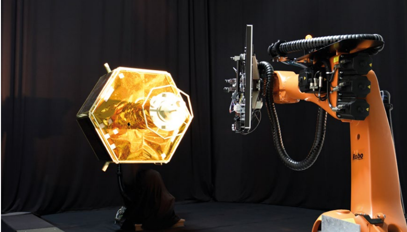
Fig. 2-5 Possible setup for sensor tests with pure black background: EPOS robot 2 (left) wrapped in black Molton with a mockup of a satellite and with Molton curtain in the background and EPOS robot 1 (right) with sensors on its adapter plate.
