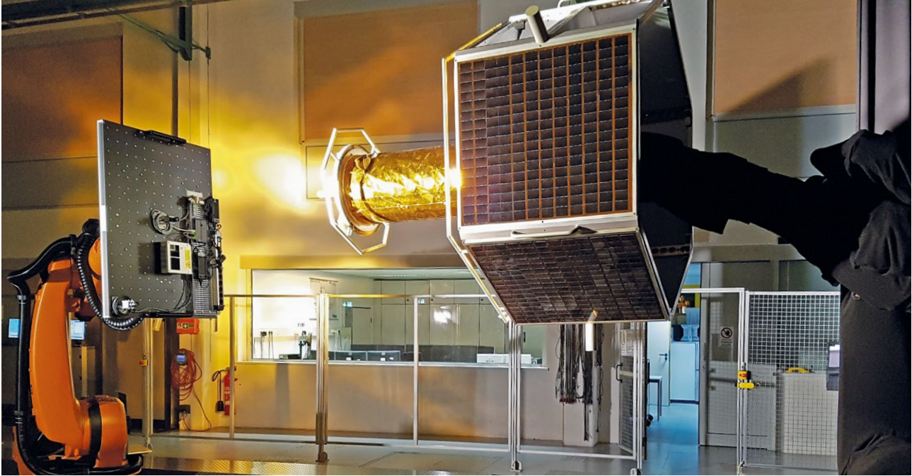
Fig. 2-1 The European Proximity Operations Simulator (EPOS) 2.0 - Facility for testing autonomous guidance, navigation and control systems for rendezvous and inspection missions
