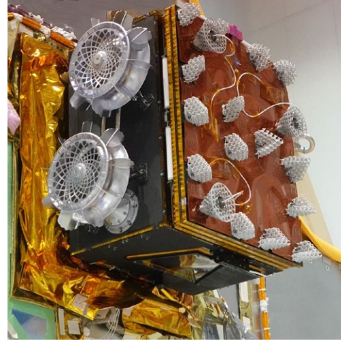
Fig. 6-2 Flight Model of IDEFIX, in stored configuration, as attached to the mothership, during cruise, before separation
