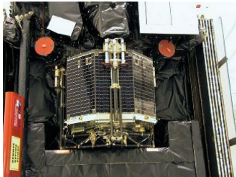
Fig. 3-3 Philae as mounted on Rosetta spacecraft in cruise configuration
