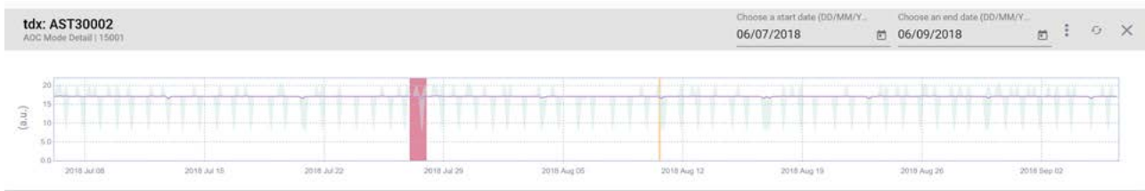
Fig. 1-2 ViDA highlighting novelties in telemetry. The bars mark the time ranges in which novelties occurred. The color indicates the severity of a novelty.
