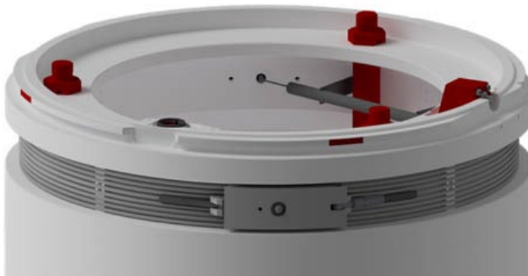
Fig. 5-6 Separation System with included YoYo-De-Spin. The flange on this module represents one side of the Manacle ring joint, whereas the round red actuators are the plungers that are pneumatically activated to separate the stages.
