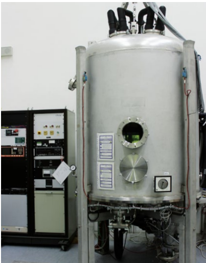
Fig. 7-3 MORABA thermal vacuum chamber
