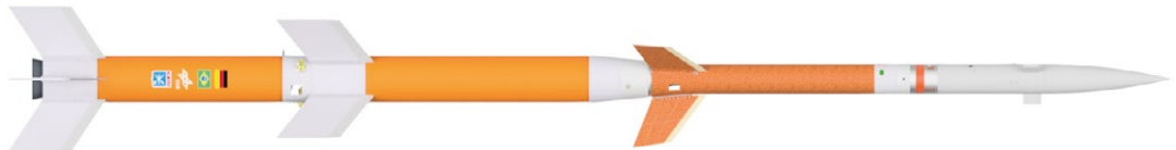
Fig. 5-5 STORT Vehicle, showing multiple stages with fins
