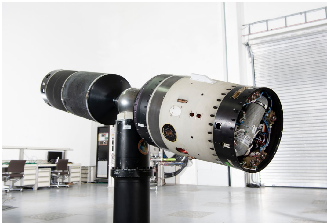
Fig. 7-5 3-D air bearing test for the verification of Cold Gas System control loops
