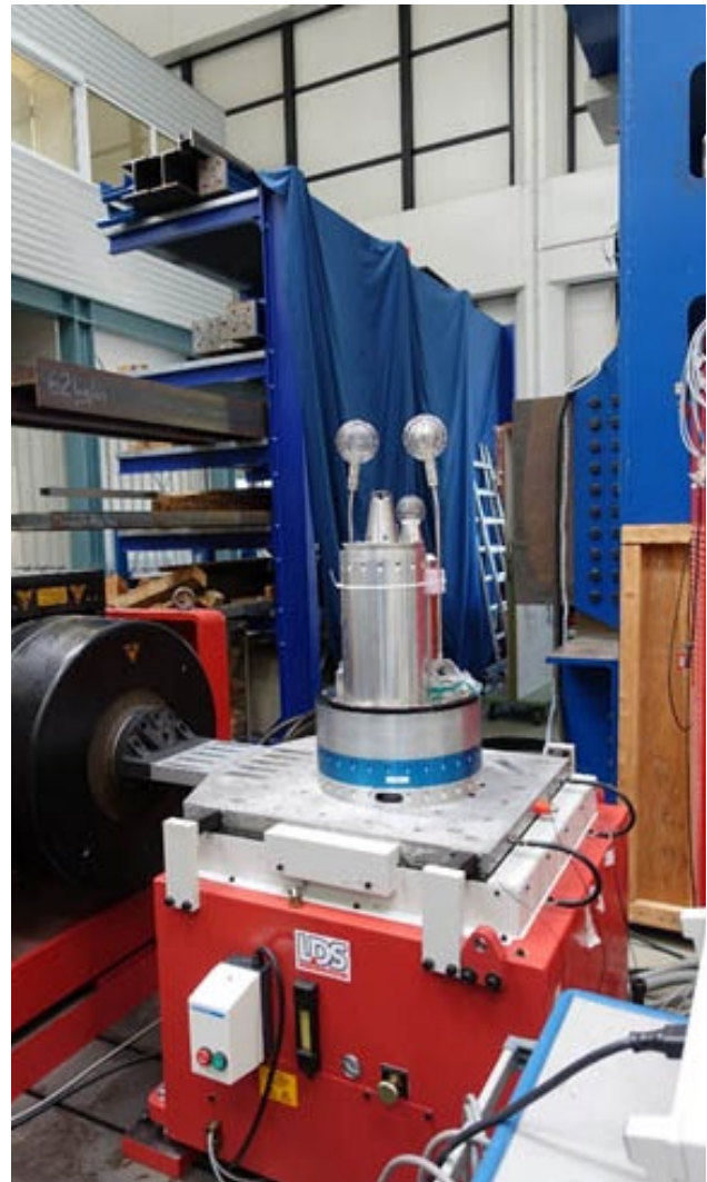
Fig. 7-4 Vibration test run of complete payload (left) and single experiment deck (right)
