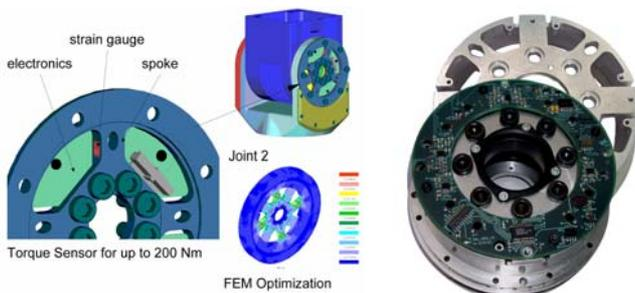
Fig. 9 FEM calculation and real torque sensor
