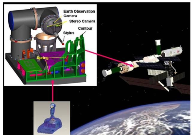
Fig. 1 ROKVISS manipulator with the contour following environment
