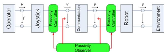
Fig. 13 Control Scheme for Time Domain Passivity Control
