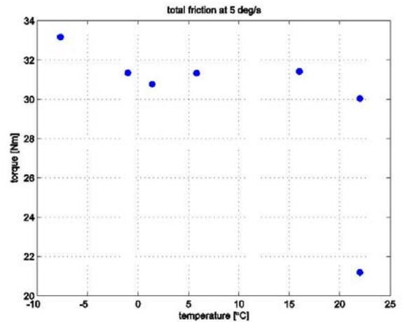
Fig. 22 Total friction at 5deg/s, plotted over the temperature. The isolated value corresponds to the reference measurement on ground.
