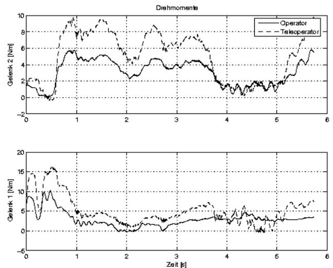
Fig. 16 Recorded torques during telepresence contour following
