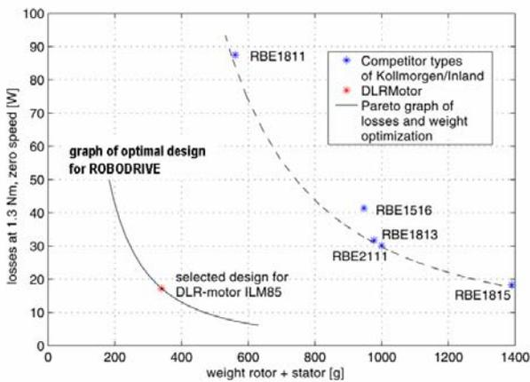
Fig. 8 Comparing ROBODRIVE with the best commercially available motors
