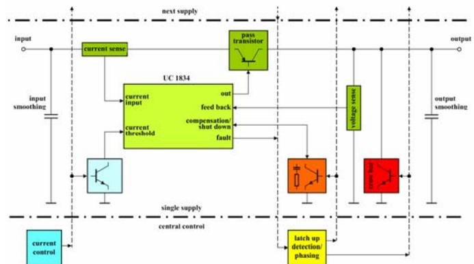
Fig. 10 The new latch-up protection circuit
