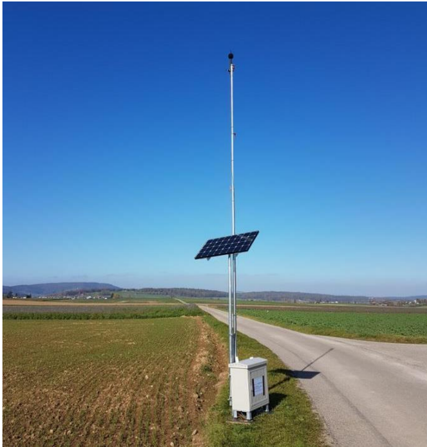
Figure 2: Example of a mobile measurement station consisting of microphone, solar panel and measurement cabinet.
