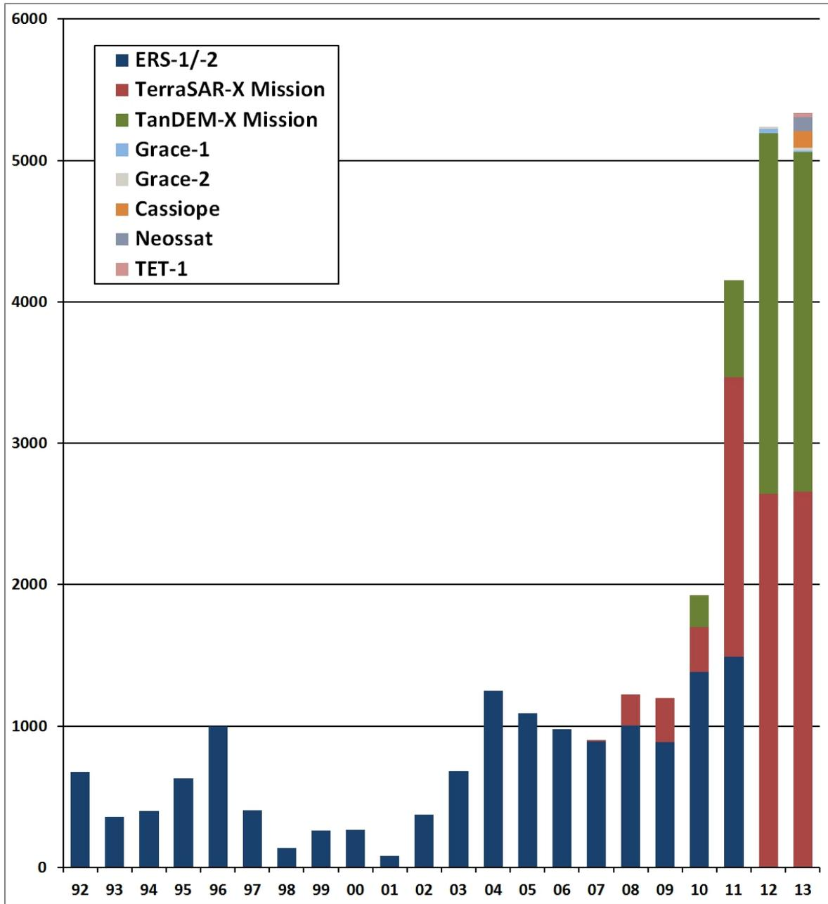
**Fig. 3.** Data acquisition at GARS O'Higgins. All contacts from 1992 to 2013 are shown. They include payload data reception, TT&C and LEOP support. ERS-1/-2 contact only took place during defined campaigns during the Antarctic summer.
