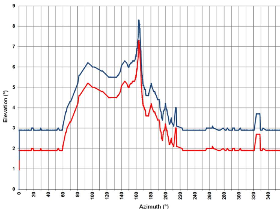
**Fig. 2.** Currently used elevation mask of the OHG antenna for S-band (red) and X-band (blue), which guarantees good receiving quality.
