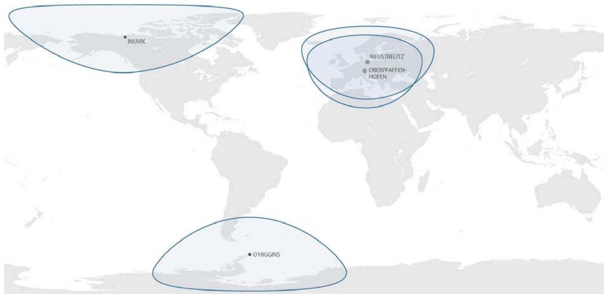
**Fig. 1.** Ground Station Network of the German Remote Sensing Data Center (DFD) of DLR. The blue circles delineate the visibility circles of the receiving stations.
