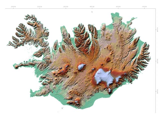
Fig. 4: Color shaded version of TanDEM-X PolarDEM 90 of Iceland
