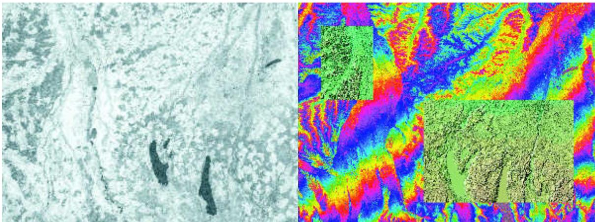
Coherence map at left and interferogram at right, the latter superimposed with two segments of a digital elevation model.
