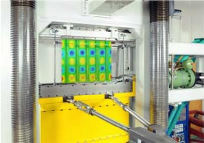
Fig.2: Panel under axial compression load
