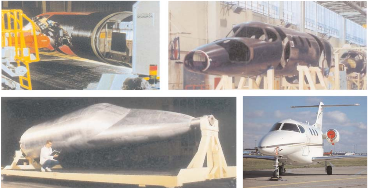
Fig. 3. Carbon fiber fuselage of the light passenger airplane Premier I
