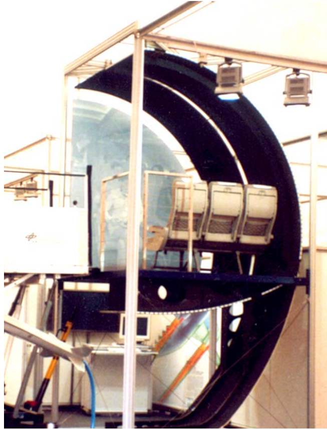
Figure 9: Full scale CFRP Fuselage Demonstrator
