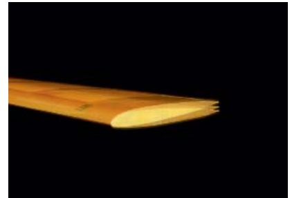
Fig. 1: Amplitudes of \pm 2^\circ at the tip of the active twist blade.
