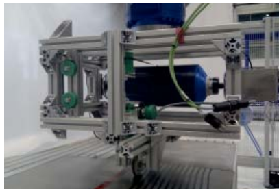
Fig. 2: Experimental Fiber Placement Head.
