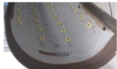
Fig. 3: Implementation of SHM sensor network for the Tailboom.
