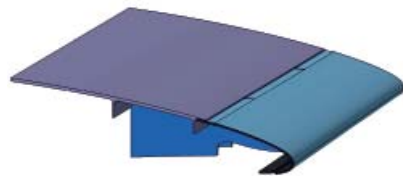
Fig. 2: Floating Lap Joint design for nose – wing upper cover interface.
