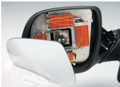
Fig. 3: Rear-view mirror with the first proto-type of the double spiral isolation interface.
