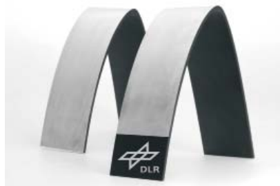
Fig. 3: Integration of metal sheets and elastomeric material in leading edge for erosion protection.
