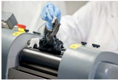
Fig. 1: Dispersing of CNTs in an epoxy resin on a three-roller mill.
