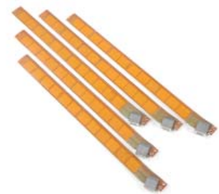
Fig. 3: Complete set (4 + spare blade) of fully instrumented rotor blades for wind tunnel tests.
