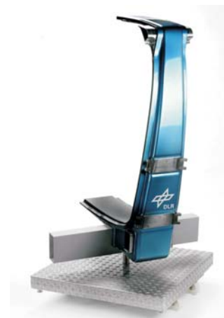
Fig. 2: Composite B-Frame replacing B-Pillar.
