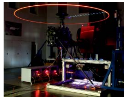
Fig. 2: Test of a single active twist blade on a rotor test rig.
