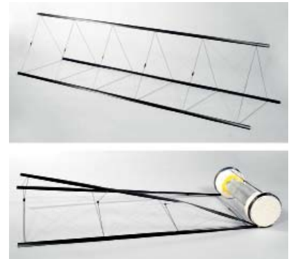
Fig. 1: Truss prototype of 0.35m radius in deployed and semi-folded state.
