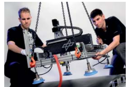
Fig. 2: Mounting of Automatic Repair Unit on a curved composite structure for repair.
