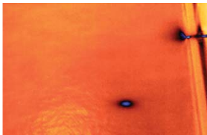
Fig. 2: Surface leakage and leakage at the sealing tape.
