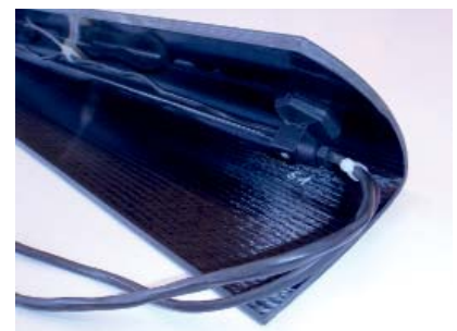
Fig. 2: Rear view of the laminar leading edge with a combined electrical connector for power supply and sensor data.
