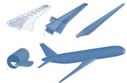
Fig. 2: Modularity: Wing created as beam model and shell models (upper row), aircraft as segments and whole aircraft (lower row).
