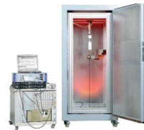
Fig. 2: Current test stand with control box (left) and acoustic-isolated chamber (right).
