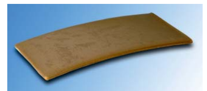
Fig. 2: Demonstrator sandwich panel made of flax fiber reinforced top layers and flame retardants (A380 hat rack, scale 1:2).
