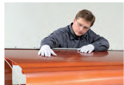
Fig. 6: Large scale droop nose section (side view) with marked high lift contour.
