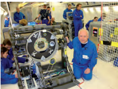
Fig. 3: Test rack with stowed antenna on board the NOVESPACE Zero-G aircraft.
