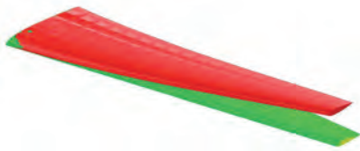
Fig. 1: Global deformation of a wing under aerodynamic loads.
