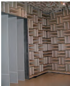
Fig. 2: Anechoic room of the test facility.
