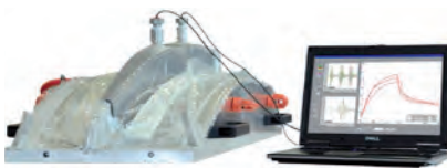
Fig. 2: Frame tool with vacuum assembly and integrated sensors.
