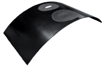
Fig. 1: Demonstrator of a hybrid RFI-infusionsrepair.
