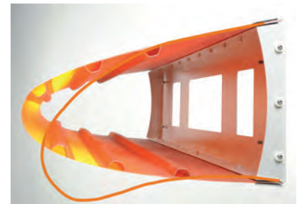
Fig. 6: Large scale droop nose section (side view) with marked high lift contour.
