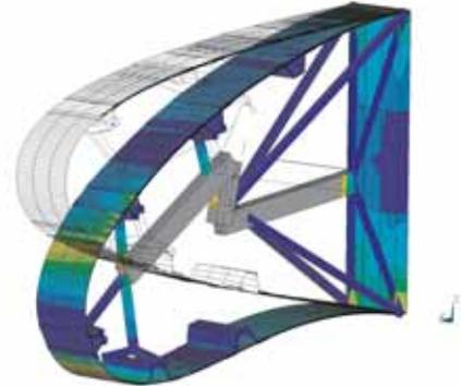
Fig. 5: Virtual proof of concept by detailed finite-element analysis featuring skin, stringers and driving kinematics.
