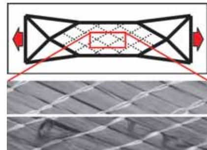
Fig. 1: Bias extension test schematic, examples for effects of shear deformation on quality of different NCF textiles.
