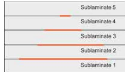
Fig. 1: Cross section of a damaged laminate: Four stacked delaminations (red lines) split the laminate into five sublaminates.
