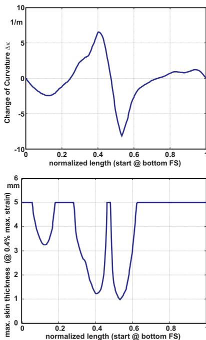
Fig. 2: Local change in curvature along normalized skin perimeter (a, top); resulting thickness from theoretical analysis (b, bottom).
