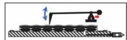
Fig. 3: Schematic of dry textile waviness measurement.
