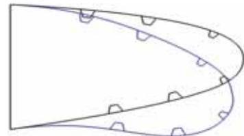
Fig. 4: Schematic stringer position layout in clean and deployed configuration.
