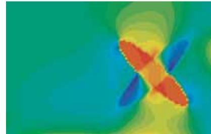
Fig. 2: Stress in fibre direction in the middle of the topmost ply of a damaged composite laminate. The laminate is loaded compressively in vertical direction. The elliptical shape of two delaminations is clearly reflected in the stress distribution.
