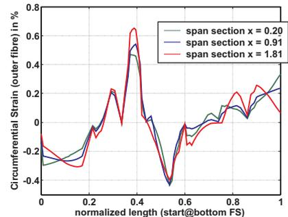
Fig. 3: Circumferential strain in outer skin layer at three different span sections vs. normalized skin perimeter length.
