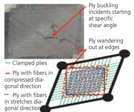
Fig. 2: Schematic of large area picture frame test with quadraxial NCF and two free moving plies.
