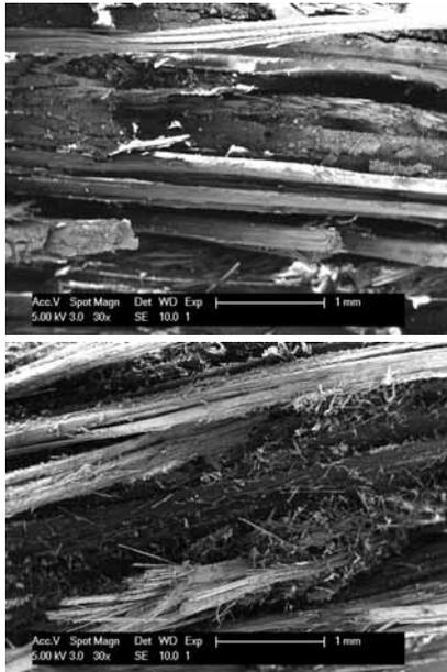
Fig. 1: Micrographs of good (upper) and insufficient (lower) fibre-resin system adhesion.
