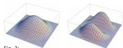
Fig. 3: Two of the six basic buckling modes used for the approximation of the sublaminates buckling shape (Ritz approach).
