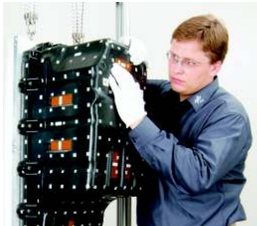
Fig. 2: Truck oil pan equipped with piezoceramic actuators.
