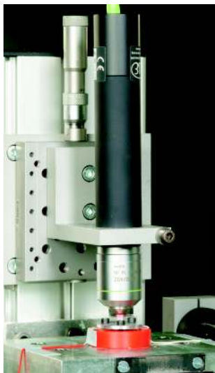
Fig. 2: Test setup for the characterization of CNT based actuators with solid electrolytes.
