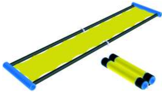
Fig. 1: Proposed membrane antenna in deployed and stowed configuration .
