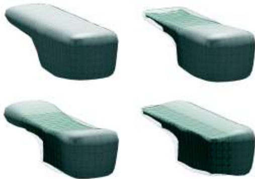
Fig. 1: Radiation filters numerically computed for truck oil pan (first top left, clockwise increasing order).
