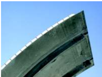
Fig. 2: CFRP design concept for sidewall, roof, and intermediate floor of composite car body.
