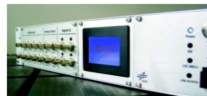
Fig. 3: PC-based control system cox including 8 input-, 4 output-channels and touch screen.
