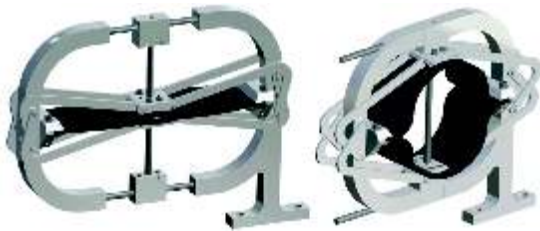
Fig. 2: Boom to spacecraft interface in closed and opened configuration.
