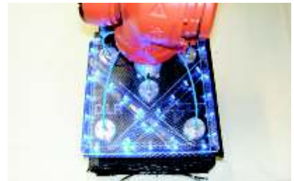
Fig. 2: End-effector with floating suction pads.
