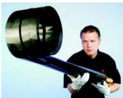
Fig. 3: Prototype of a hybrid inflatable/deployable CFRP boom for deployable space structures.
