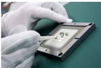
Construction of a thermoelectric module for vehicle application (TEM)
