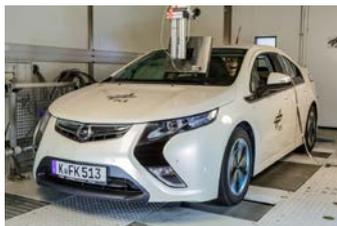
Experimental hybrid vehicle on the institute's all-wheel roller test bench
