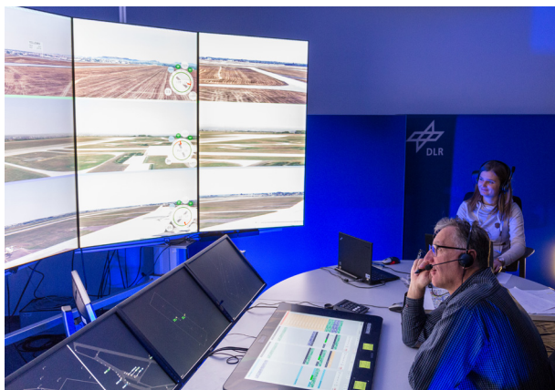
Multiple remote tower setup for three airports
