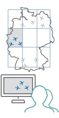
The Sectorless ATM concept with aircraftcentred ATC (left) in comparison with conventional sectoring (right).
