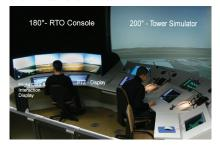
Simulation experiment in an RTC environment with two simultaneously controlled regional airports.
