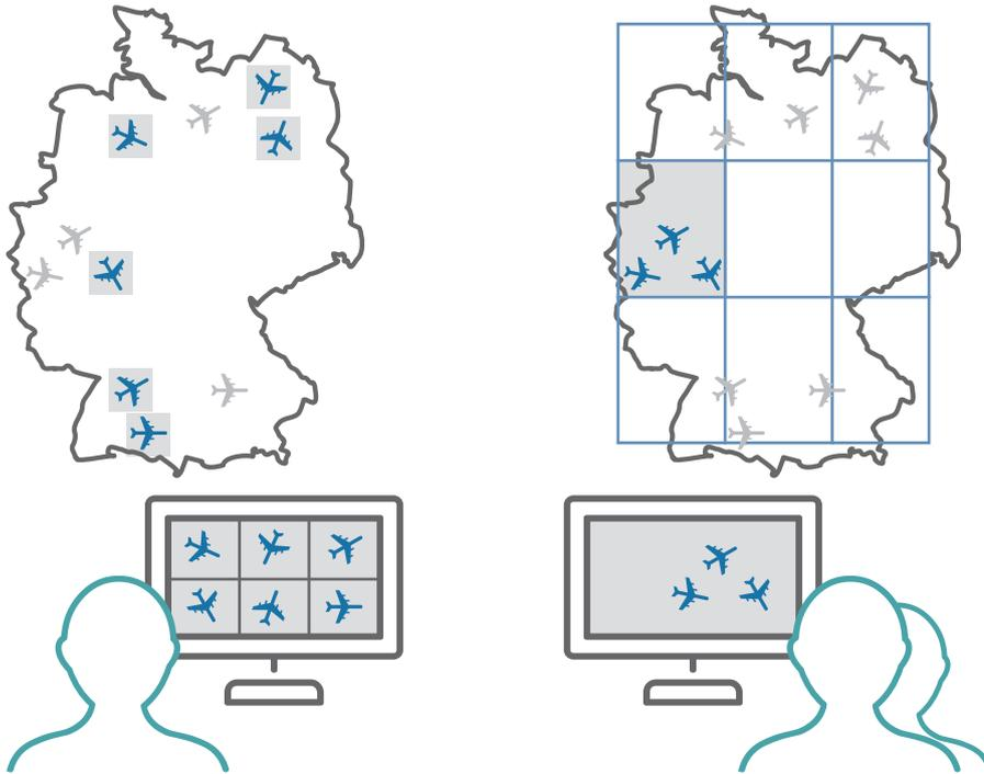
The Sectorless ATM concept with aircraft-centred ATC (left) in comparison with conventional sectoring (right).
