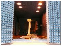
The CTR system is assembled inside a shielded, anechoic chamber of 24 x 11.7 x 9.7 meters.
