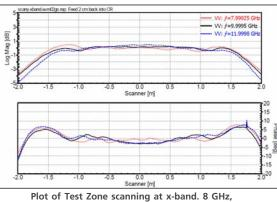
10 GHz and 12 GHz. Amplitude and Phase.
