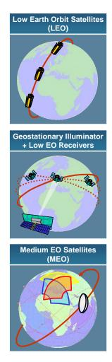
Concepts for a future constellation of radar satellites for quasi-continuous monitoring of the Earth. Top: low Earth orbit (LEO) satellites, middle: geostationary Earth orbit (GEO) transmitter with LEO receivers; bottom: medium Earth orbit (MEO) satellites.
