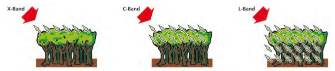
Comparison of the penetration depth in vegetation for X, C and L-band with 3 cm, 5 cm and 24 cm wavelength. While radar waves in X-band are only reflected from the upper canopy, L-band penetrates down to the ground. Only L-band radar systems can receive signals from all vegetation layers.
