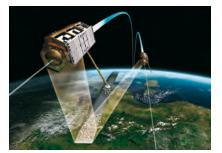
**TerraSAR-X** is the latest generation of radar satellites and was launched on the 15th June 2007 from Baikonur/ Kazakhstan. Since then, the satellite has been orbiting the Earth at an altitude of 514 km in a polar orbit. With its active radar antenna, it generates images with a maximum resolution of one meter. TerraSAR-X is Germany's first radar satellite and was realised in a publicprivate partnership between DLR and Airbus Defence and Space.
