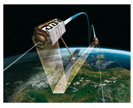
The TanDEM-X mission is the first radar interferometer in space with the controlled formation flight of two radar satellites.
