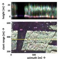
Demonstration of tomographic imaging of a group of trees in L-band. In this example, the radar data were recorded using DLR's airborne SAR system by making several passes at intervals of a few minutes.
