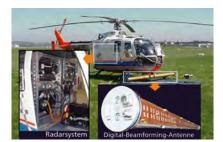
Digital beamforming demonstrator on a DLR helicopter
