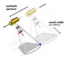
Synthetic aperture radar (SAR). The formation of a synthetic aperture several kilometers long enables a high-resolution independent of the range distance. Because of their independence of weather and daylight conditions, SAR instruments are an indispensable source of Earth observation data and enable numerous powerful applications.
