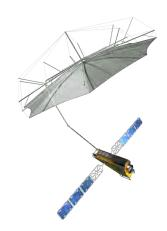
Tandem-L satellite with reflector antenna
