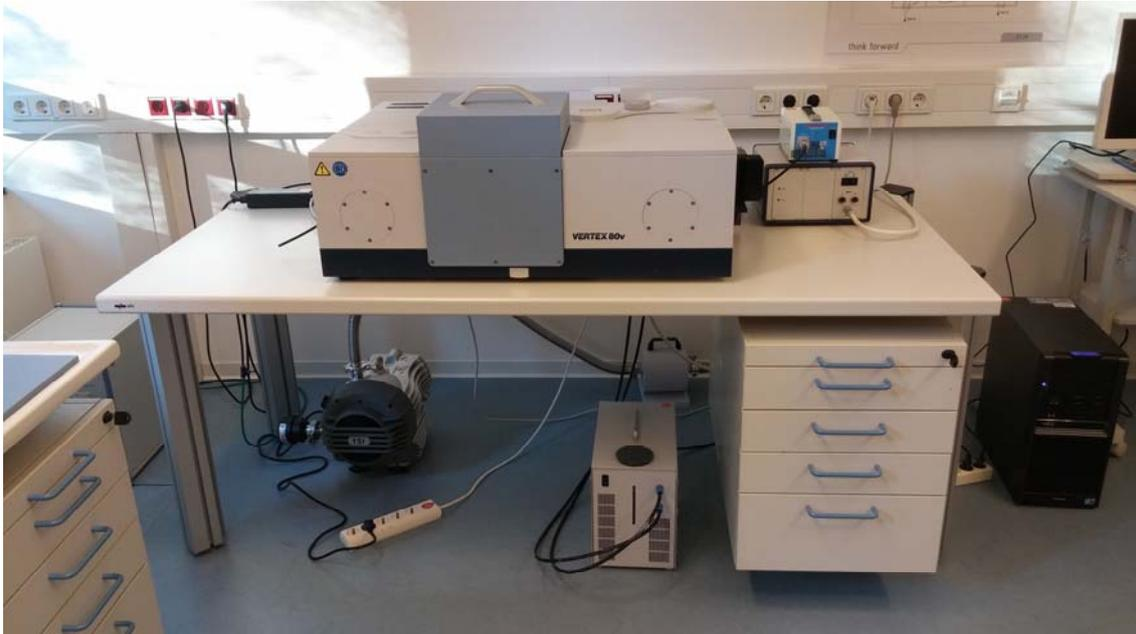
**Purpose:** Measurements of solar absorptance  $\alpha_s$ , hemispherical thermal emittance  $\epsilon_h$ , specular reflectance, and transmittance
