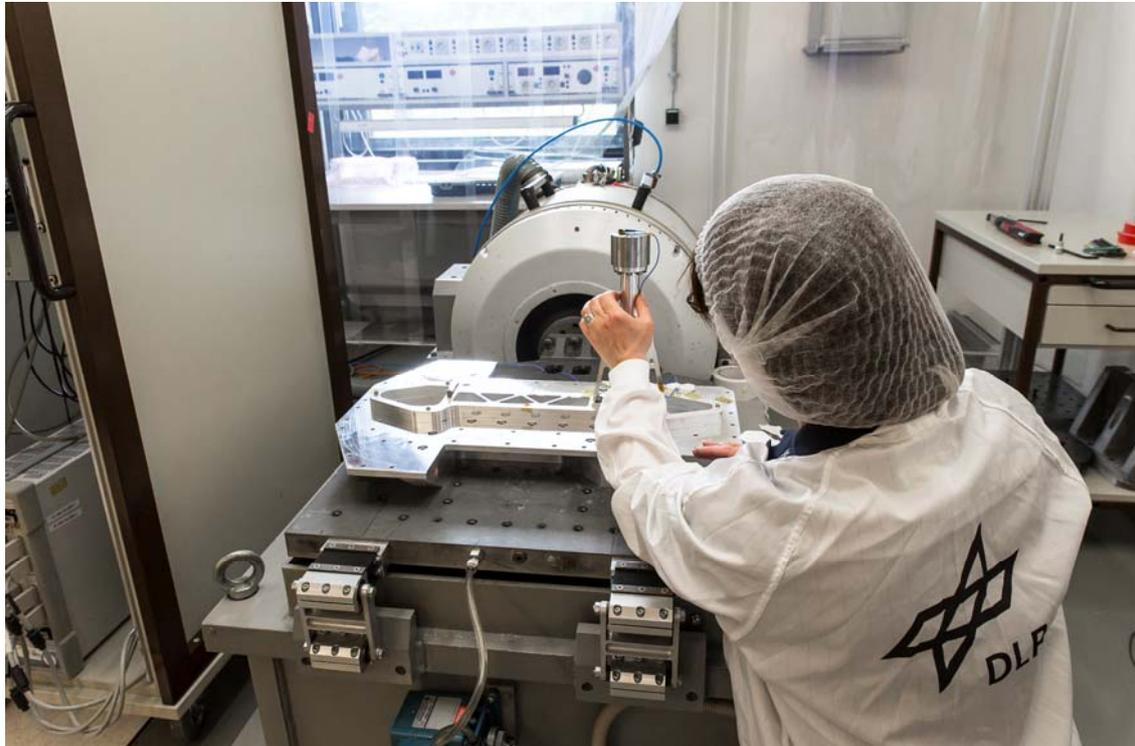
**Purpose:** Sine Vibration, Random Vibration, Half-sine Shock
