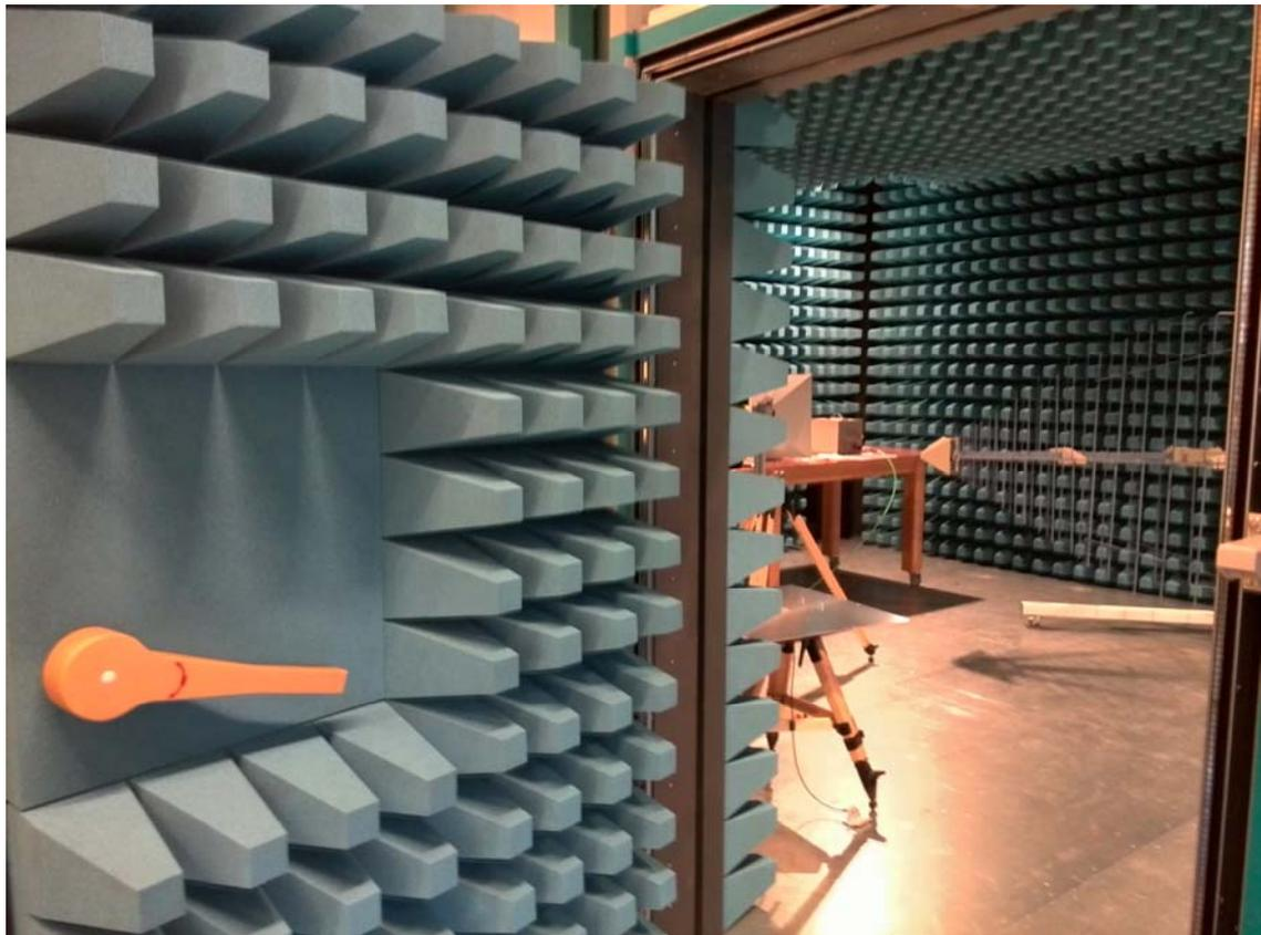
**Purpose:** electromagnetic compatibility according ECSS-E-ST-20-07C, error/disturbance detection, error/disturbance localization, DC magnetic field emission, DC magnet moment
