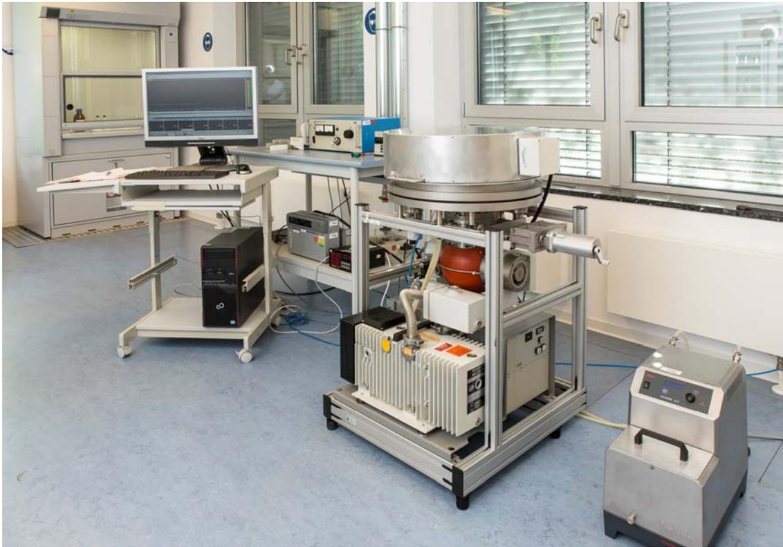
**Purpose:** Material outgassing Measurements according to ECSS-Q-ST-70-02C
