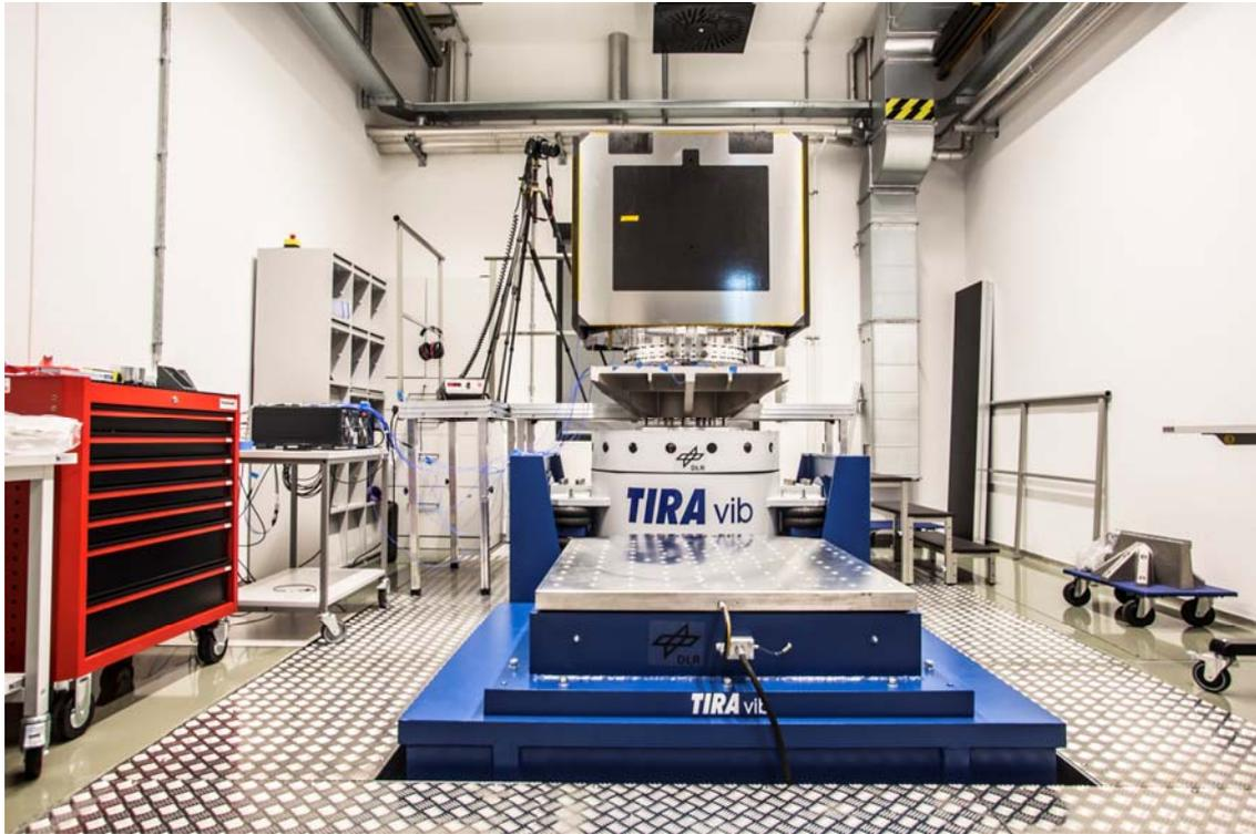
**Purpose:** Sine Vibration, Random Vibration, Half-sine Shock
