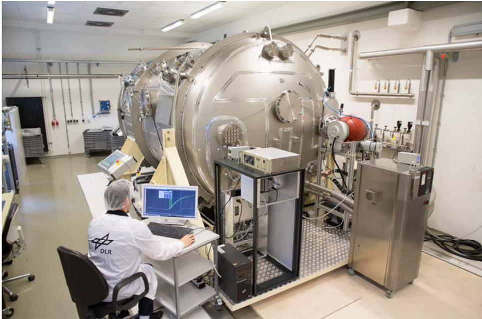
**Purpose:** Thermal Cycling with/without artificial sun, Thermal Balancing with/without artificial sun, Venting
